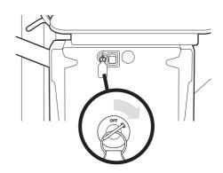
When the key and the on/off switch are in the on position, the light on the on/off switch will come on.
